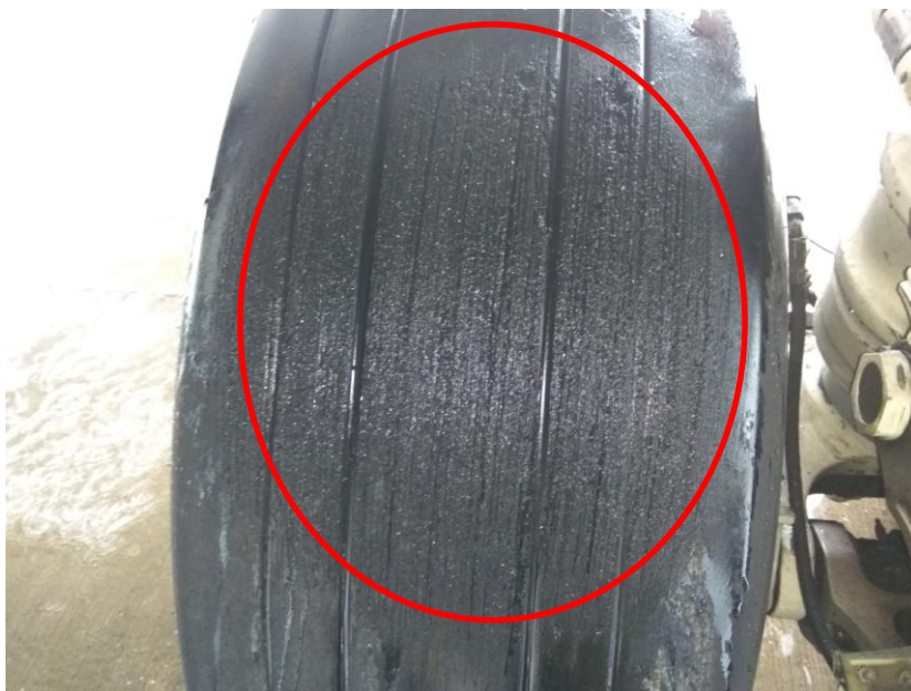
Figure # 8 Tyre # 2 worn out
