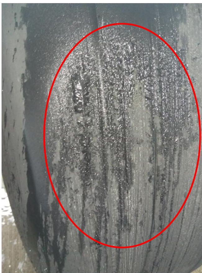
Figure # 7 Tyre # 1 worn out
