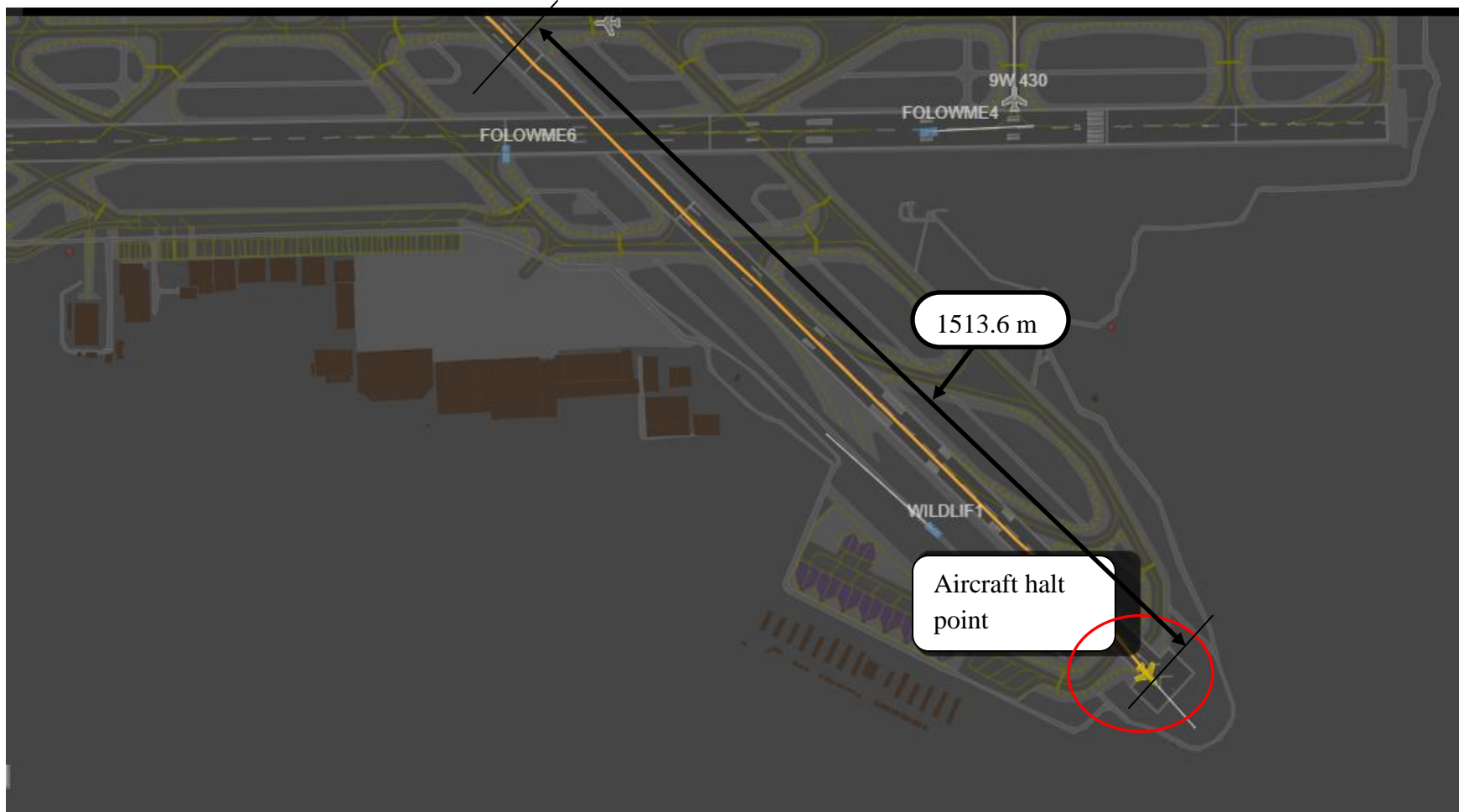
Figure # 5 IX-213 overrun the Runway 14 end and halted on paved surface after travelling 1513.6 m from touchdown
