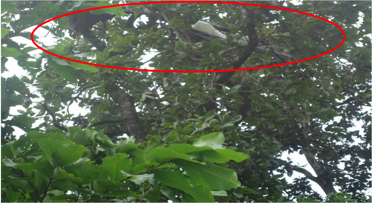
Figure 11 Red blade found hanging on the top of a tree
