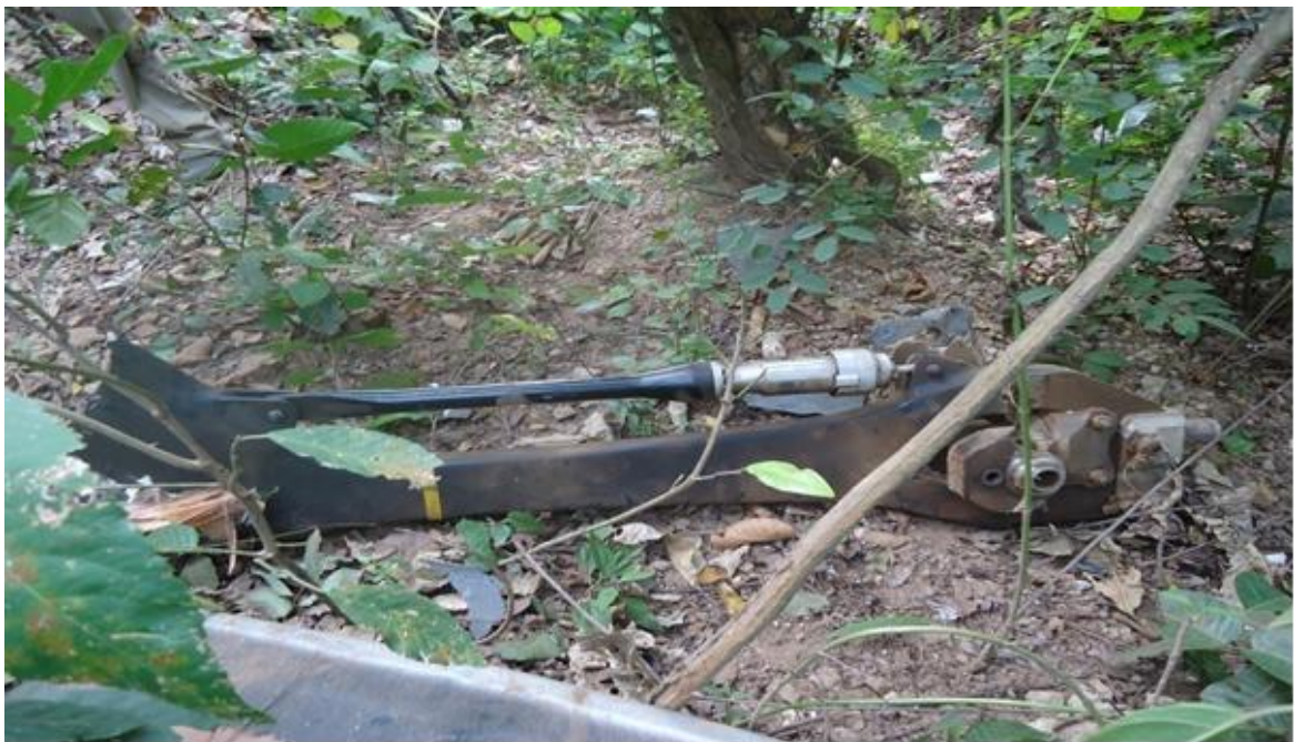
Figure 10 Yellow blade found lying at a distance of 60 m from the main wreckage
