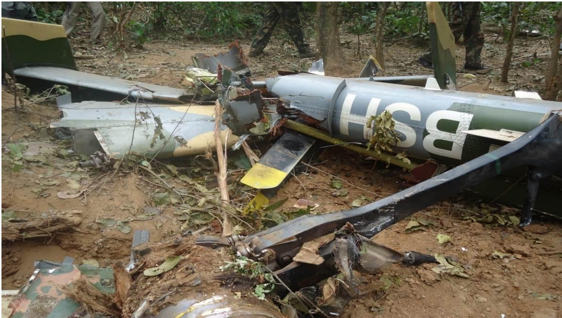
Figure 7 View of MRH with Green blade attached and un-burnt tail boom with horizontal stabiliser and tail rotor assembly
