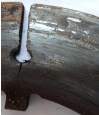
BA-15 (stator disc crack developed)
