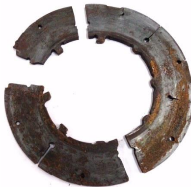
BA-16 (other stator disc in pieces)
