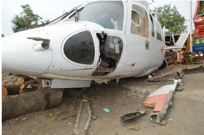
Fig:4 – Damaged Plexi window
