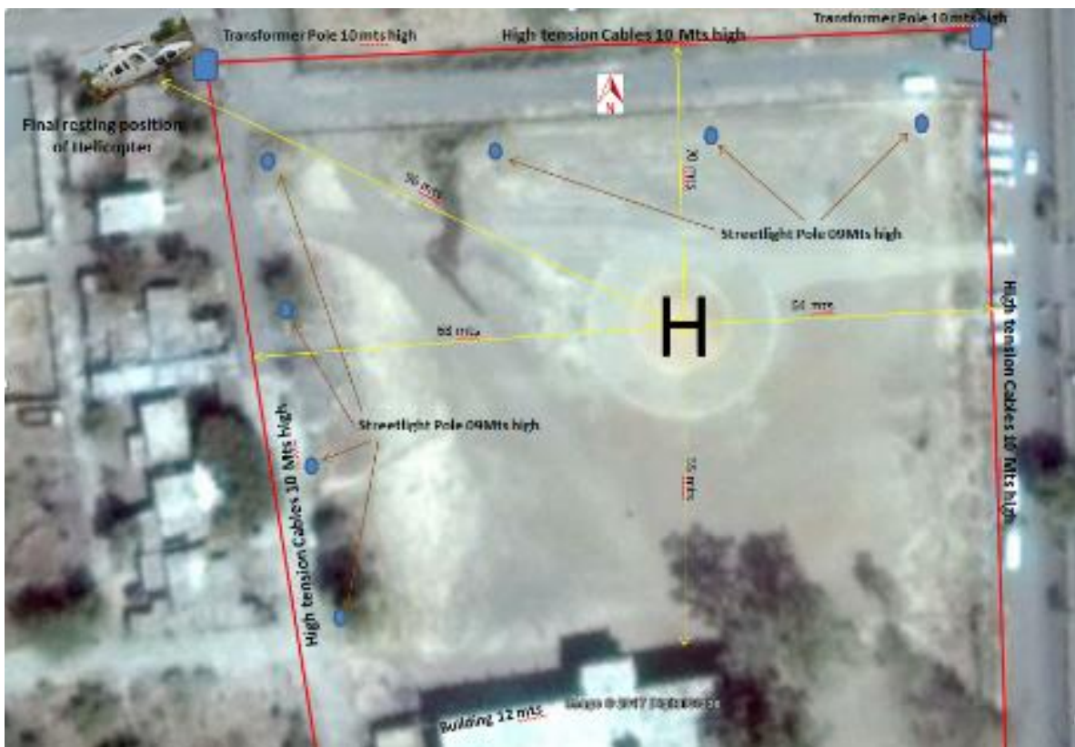
Fig:28 – Layout of the temporary landing ground.
