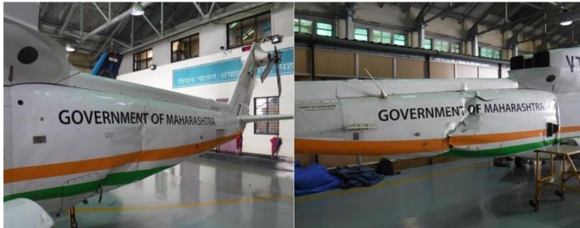
Fig:10 – Damaged Tail Section
