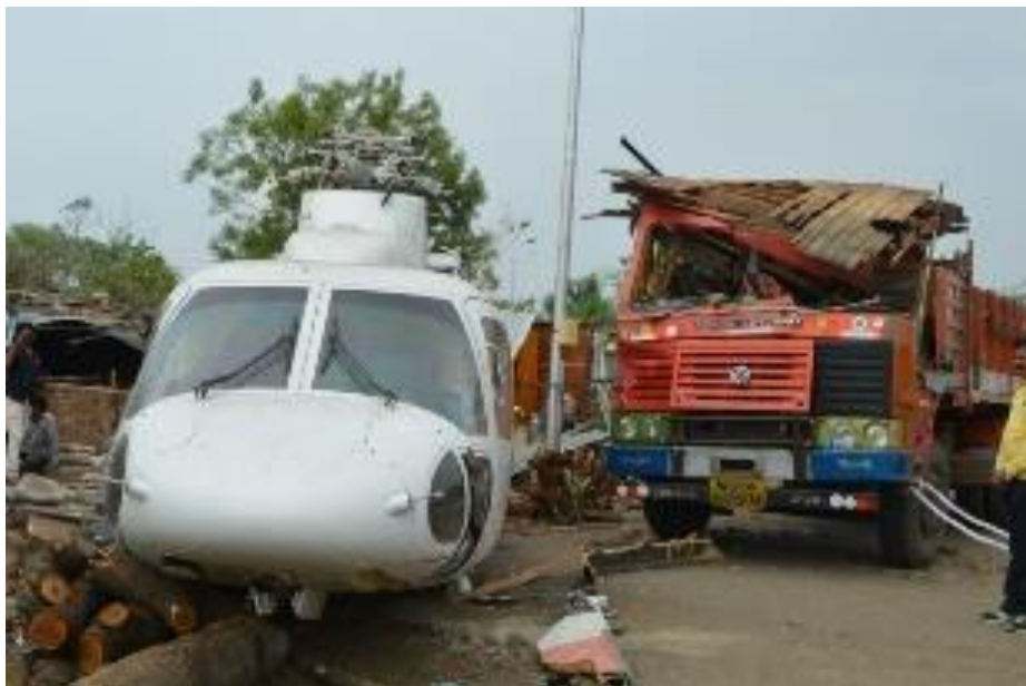
Fig:32 – Truck hit by main rotor
