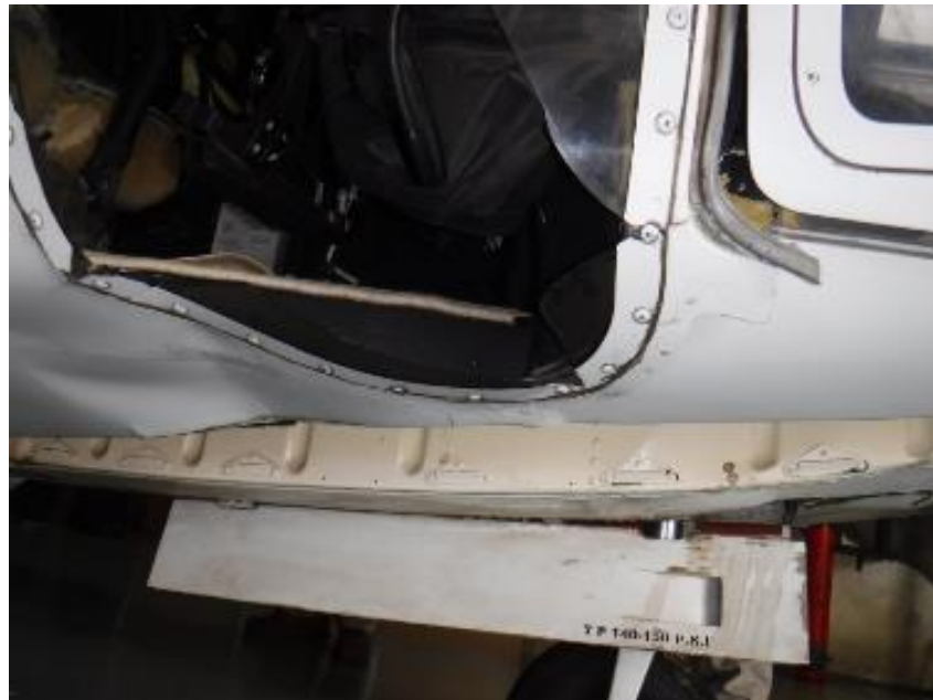
Fig:6 – RH side electronics access panel
