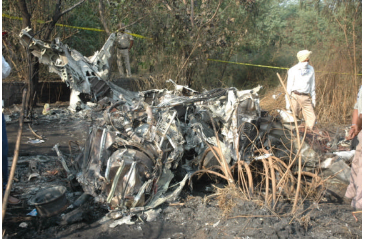
Closer view of wreckage indicating empennage, fuselage, L/G, engine, portion of right wing
