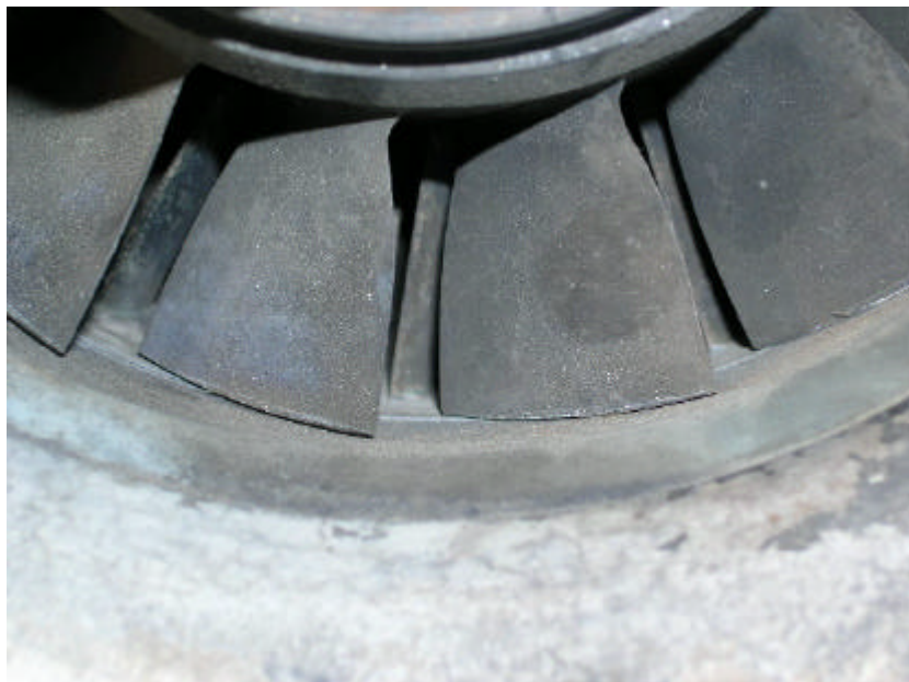
Compressor 1 st stage blades and shroud, detail.
