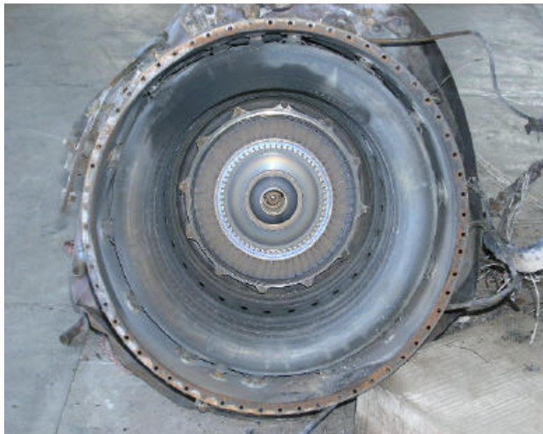
Combustion chamber liner and compressor turbine, in-situ.
