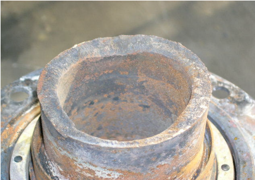
Propeller shaft, aft fracture face.
