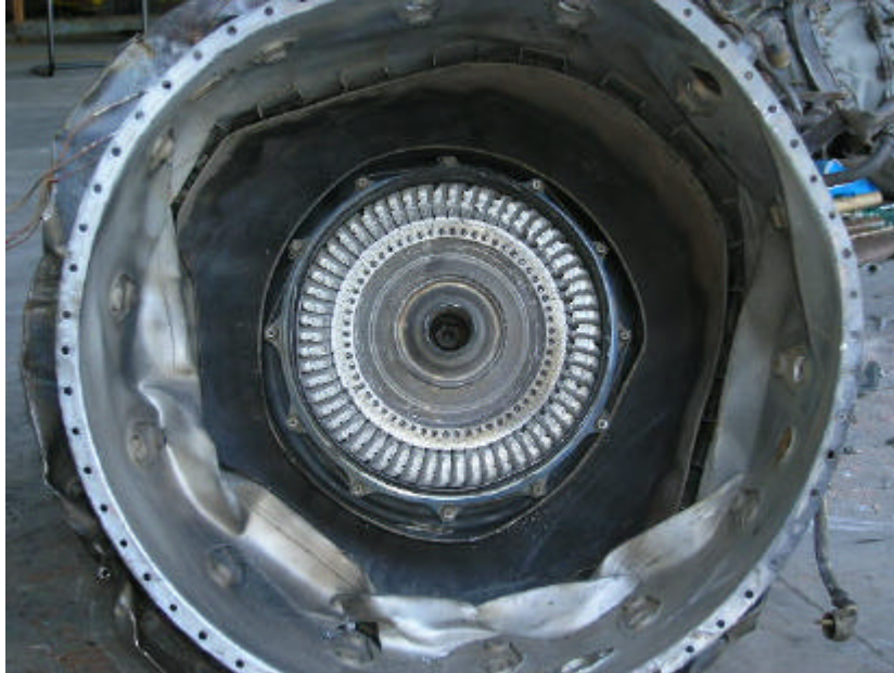
Gas generator case interior, large and small exit ducts, and compressor turbine, in-situ.
