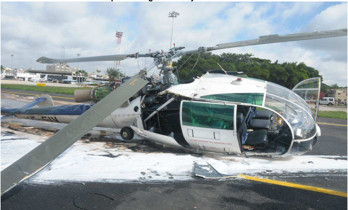
Right side view of the cockpit with right cockpit door separated
