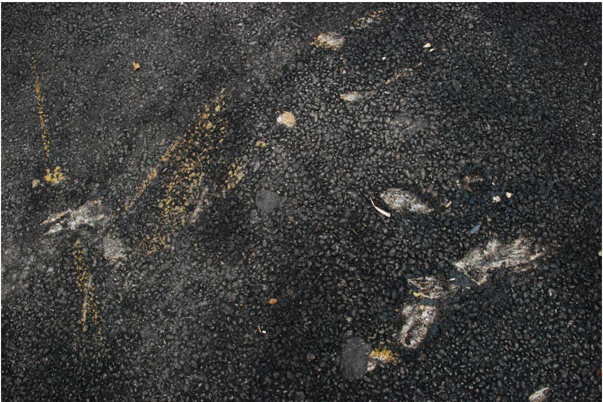
Ground marks of tail rotor guard and tail rotor blades
