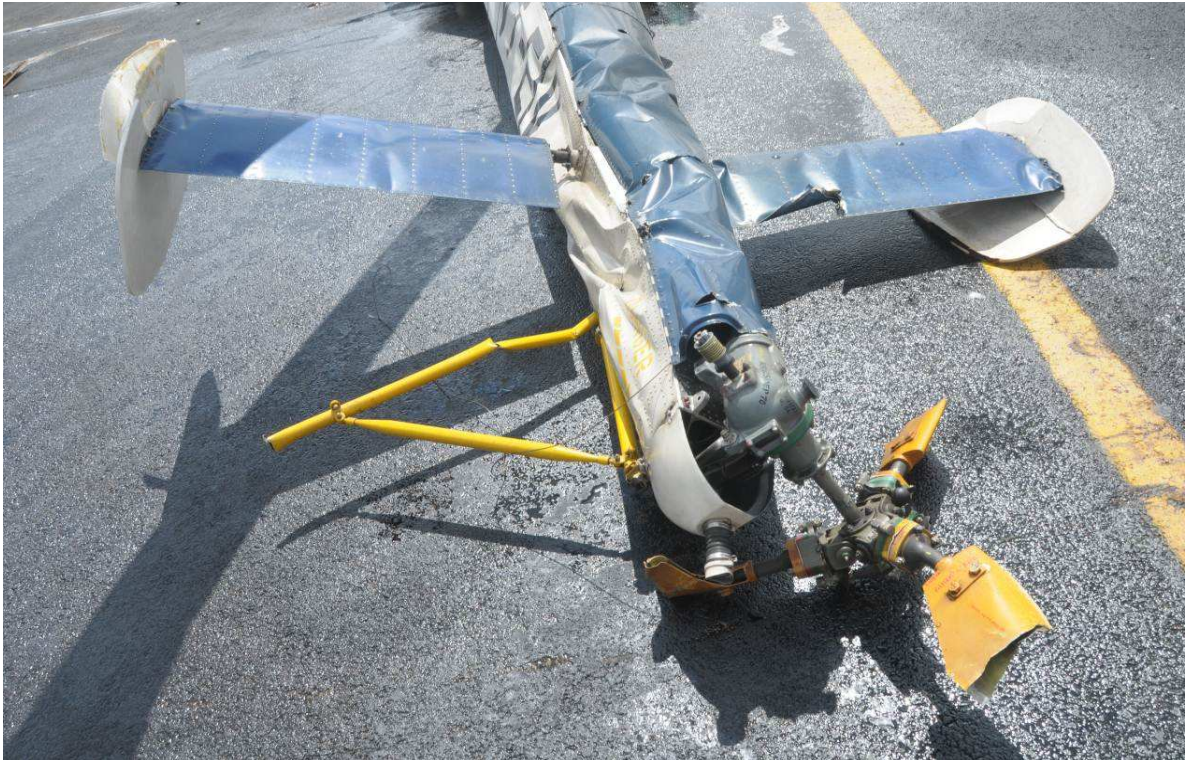
Damage to the tail rotor guard and tail rotor blades with tail boom buckled
