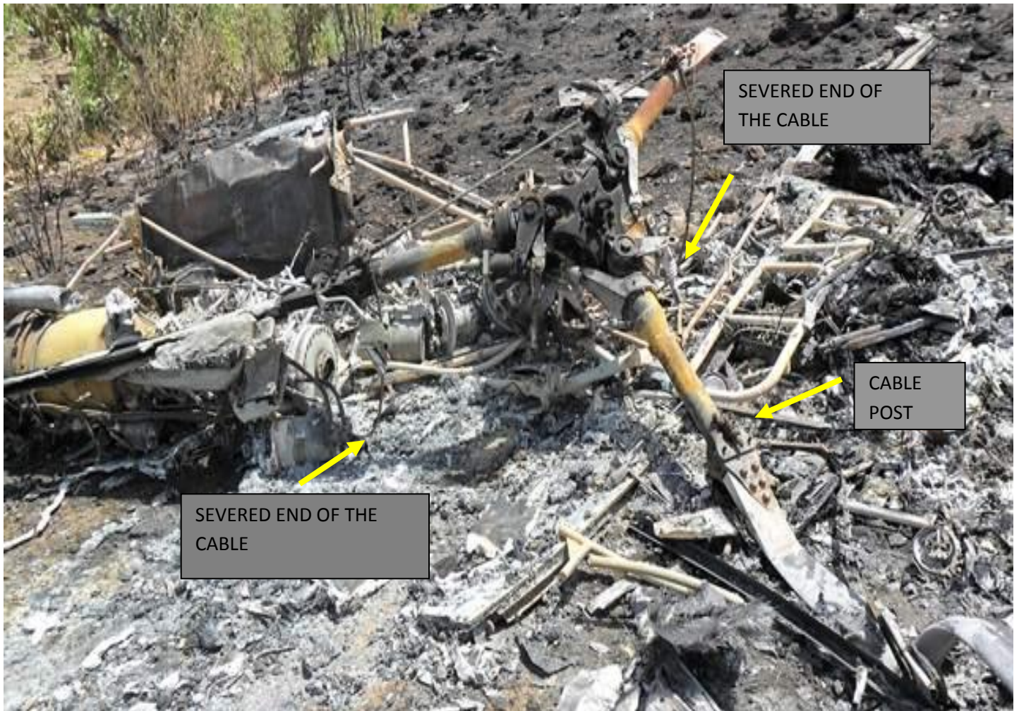
Fig-3 Main Rotor Hub Assembly with the severed spacing cables
