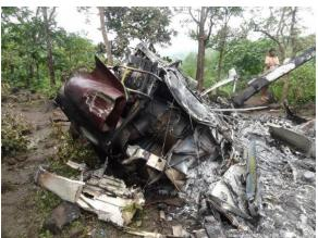
• The main rotor transmission, main drive shaft, mast, main rotor hub, blades and stabilizer bar were all found attached together lying in farther most point from the tail boom.
