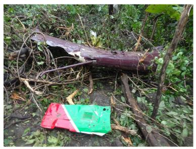
• The tail rotor hub and blade assembly were lying together at some distance from the tail boom.
