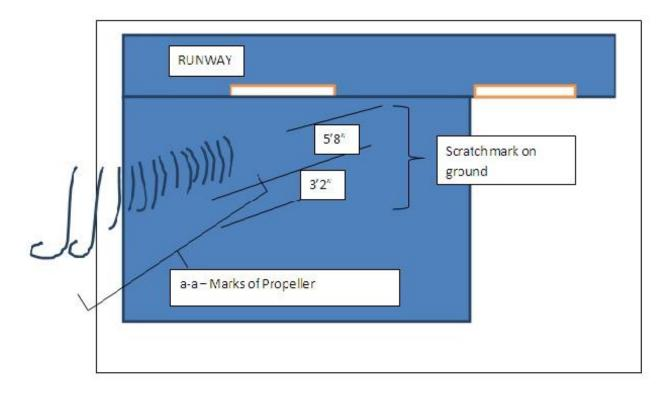
a-a : Mark of Propeller Striking the ground in running condition.
