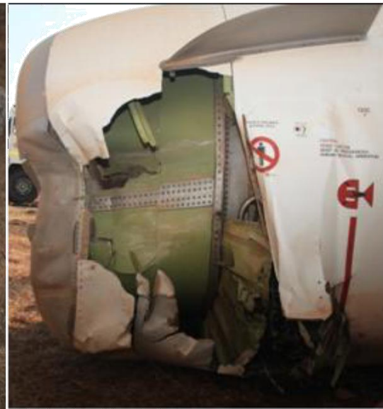
Engine damaged due hitting pillar
