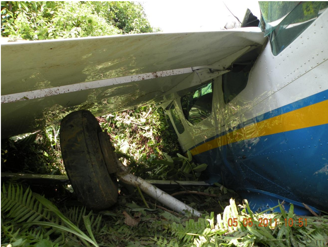
Fig-4: Broken undercarriage and caved in wing portion in the cabin.
