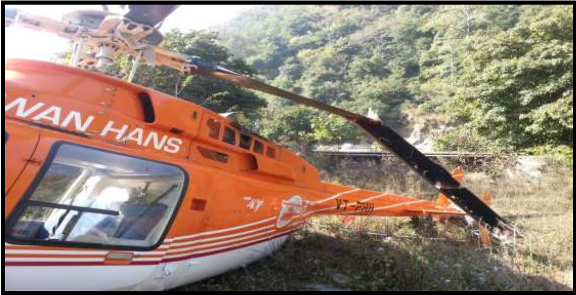
Damage to Main Rotor
