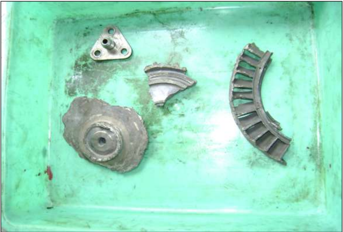
Failed 2 nd Stage Turbine
