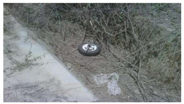
Fig. showing Right undercarriage which got separated from the aircraft after collision with the person during low-pass exercise.
