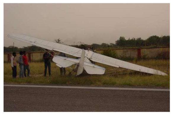
Fig showing the rear view of the aircraft with no damage to the aircraft (LH wing) and damage to right wing at the tip due scrapping & aircraft veered to the right.
