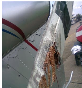
Fig. 8 Shattered TR Blade
