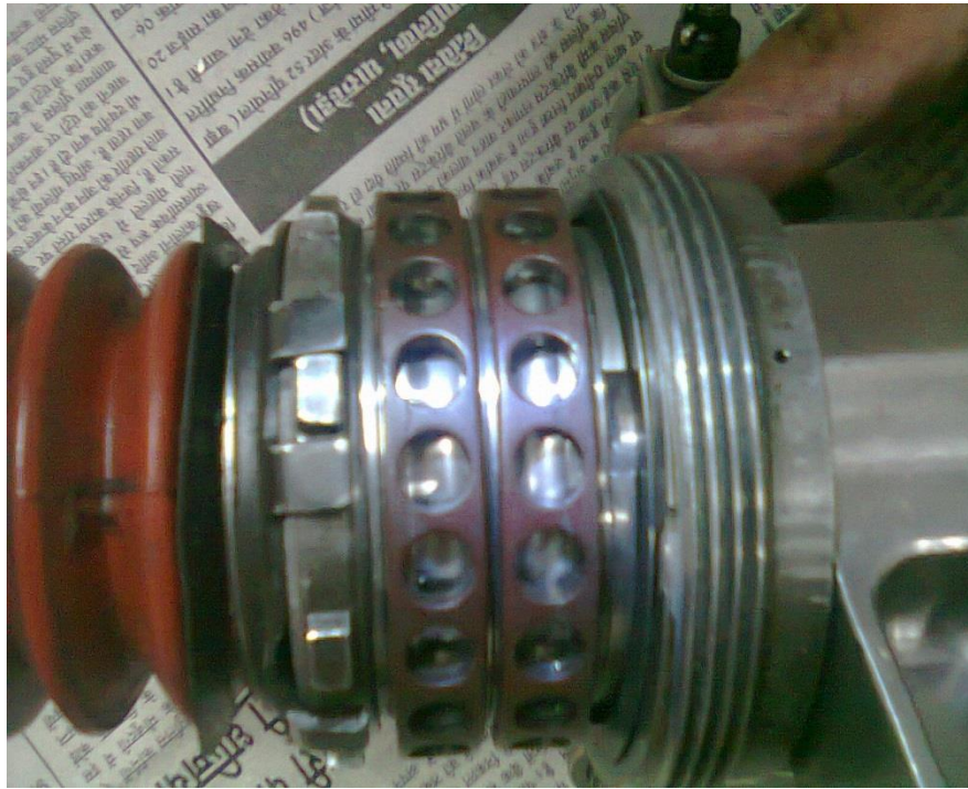
Fig. 10. Condition of Ball Bearing Holders
