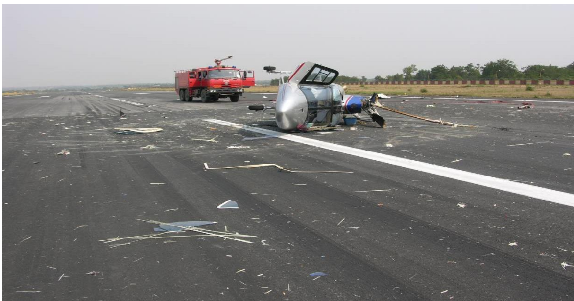
Fig. 3 MR blade marks, scattered pieces of blades & other broken parts.
