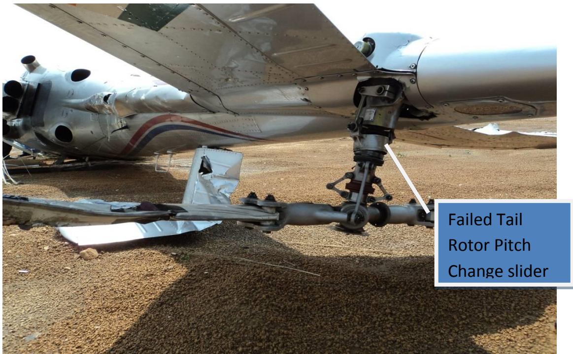
Fig.4 Failed Tail Rotor Pitch Change slider
