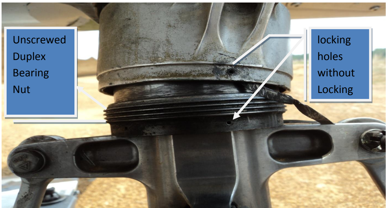
Fig.5 Unscrewed Duplex Bearing Nut & its locking holes without Locking wire
