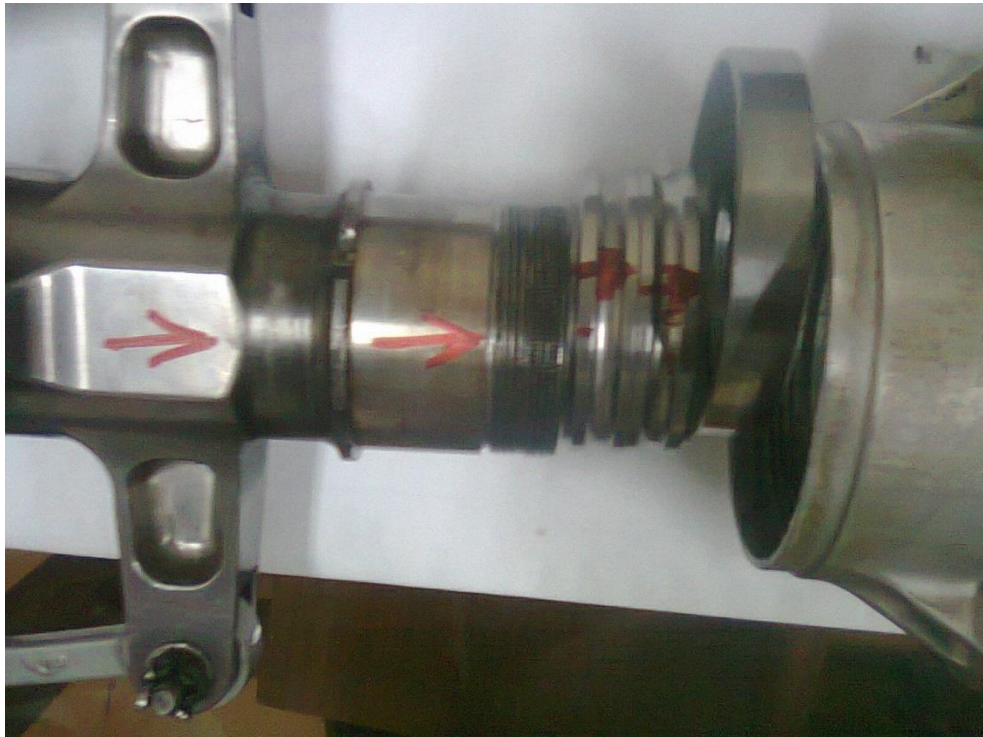
Fig. 9 Direction of inner races of Duplex Bearings
