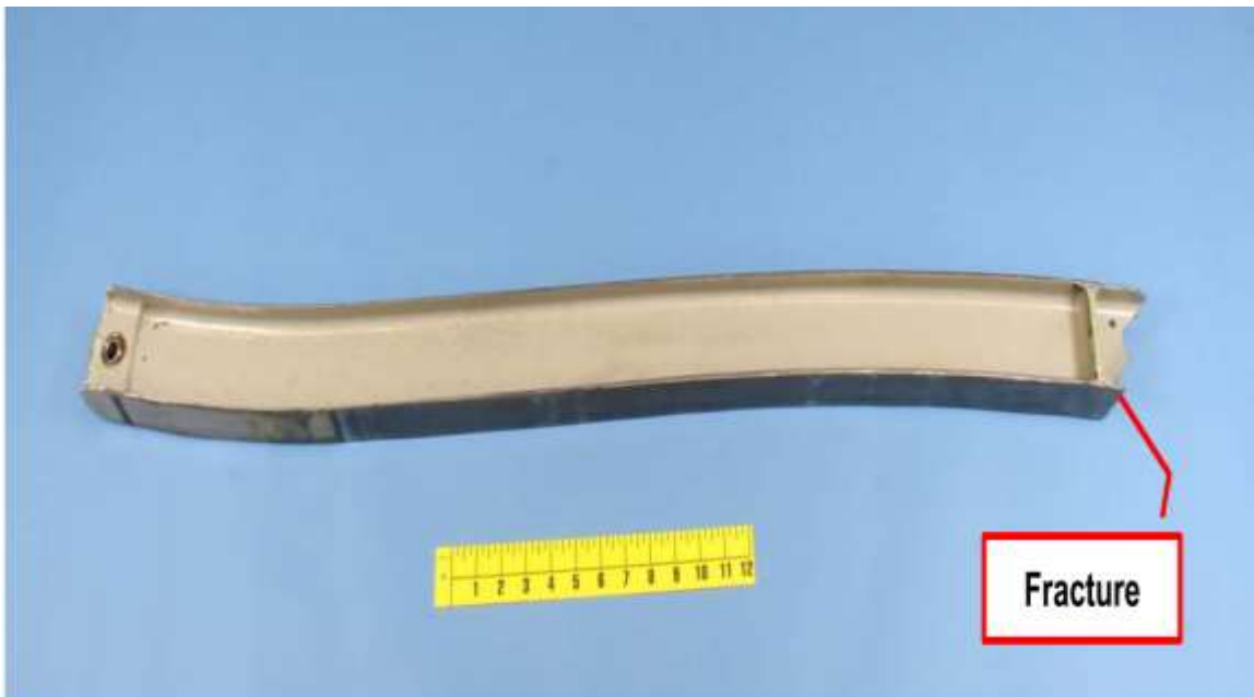
The lower flange at the aft end of the track was fractured
