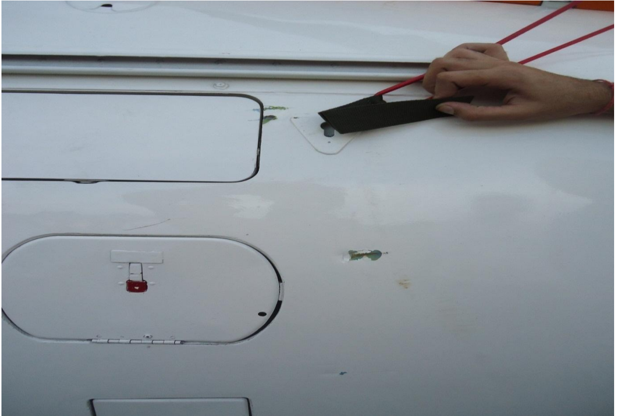
4. Small Dents and marks rear of the refueling point.
