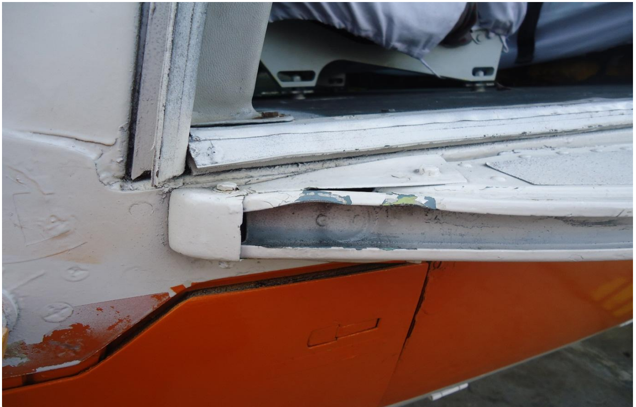
2. LH Sliding door lower rail had two curved displacement of the upper side rail near the forward end due rollers being forced through it.
