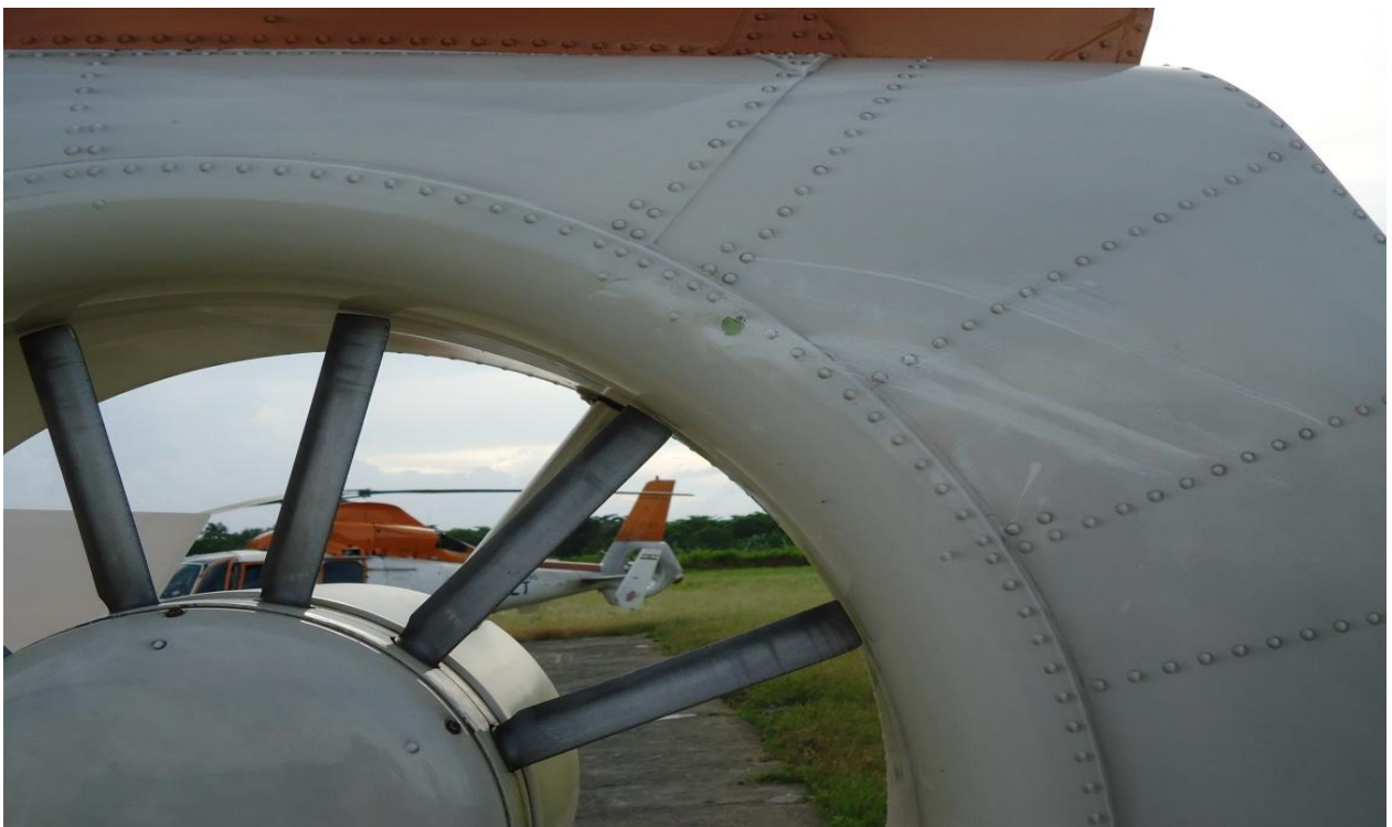
5. Small Dents and Rubbing marks over 2 O'Clock position on the Fenestron.
