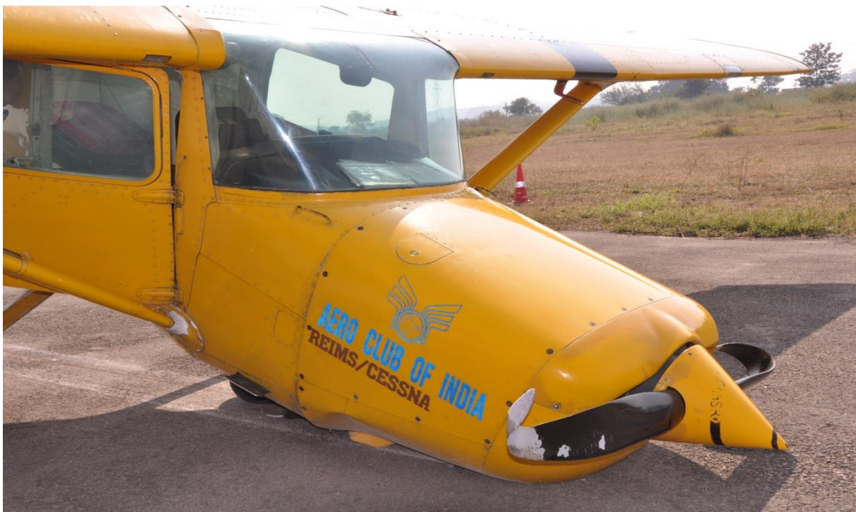
Fig.2 Showing both the propeller blades bent
