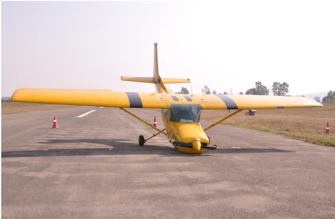
Fig.1 Showing aircraft final position veering to the left with nose under carriage collapsed.
