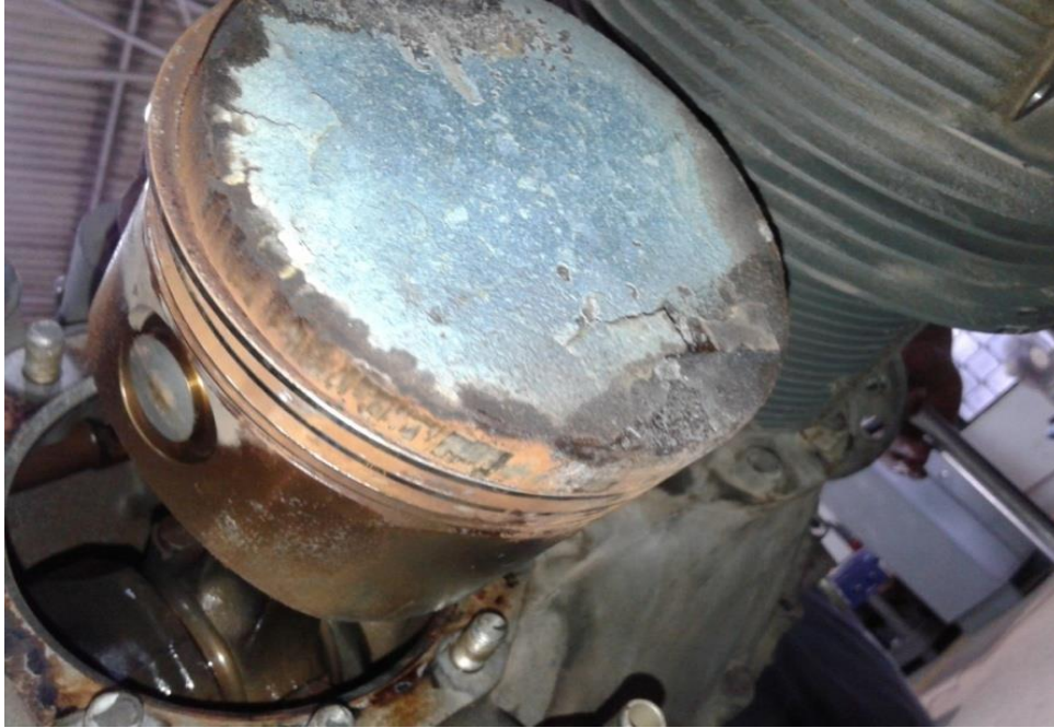
Fig 6: Piston dome (Carbon deposits noticed)
