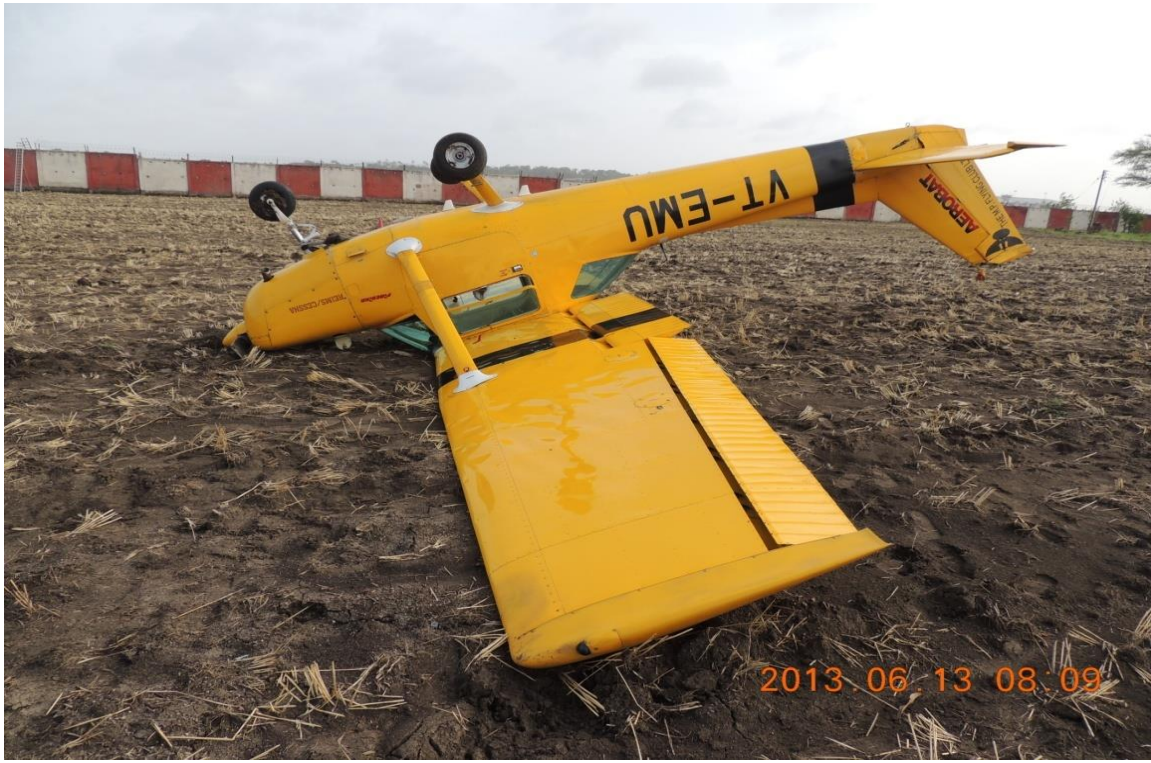
Fig: 3:-Portside wing leading edge near wingtip found damage.
