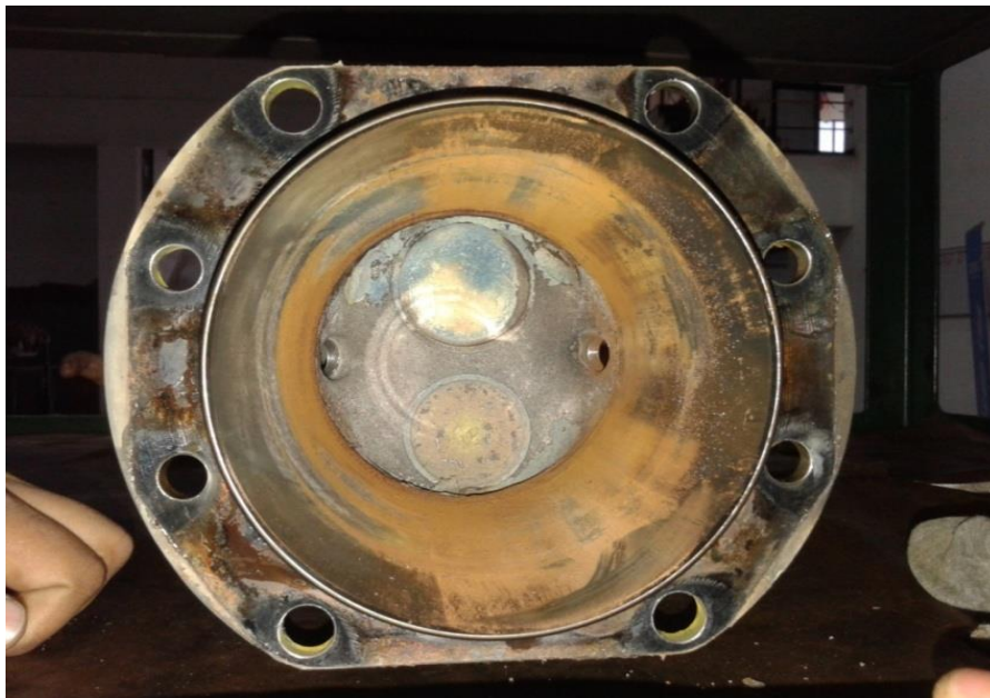
Fig 7: No. 3 Cylinder barrel (in corroded condition)
