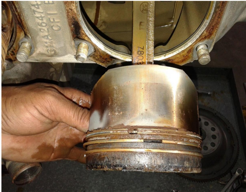
Fig 8: Condition of No.1 piston& its rings
