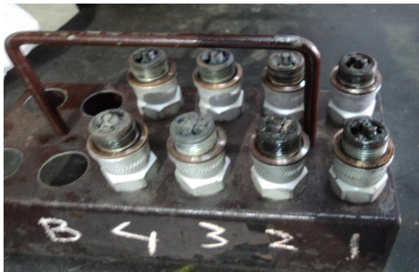
Fig 9: Condition of T(Top) and B(Bottom) Spark plugs after removal
