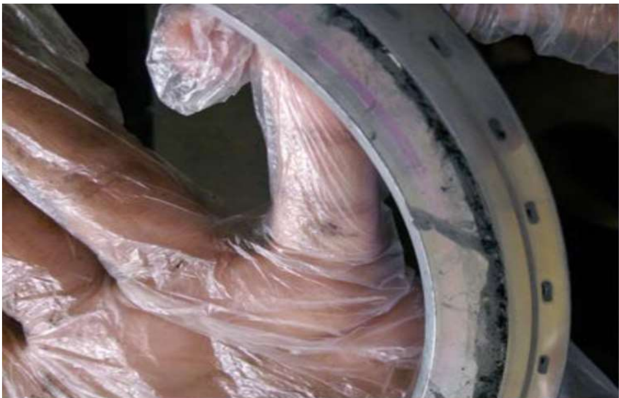
Image #6 – Post lapping condition of the demonstration seal plate.
