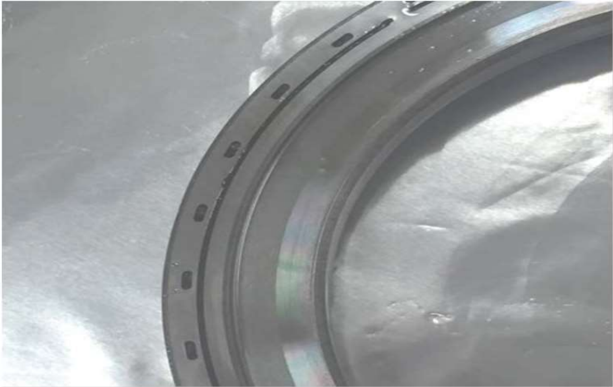
Image #7 – Post cleaning condition of the demonstration seal plate.
