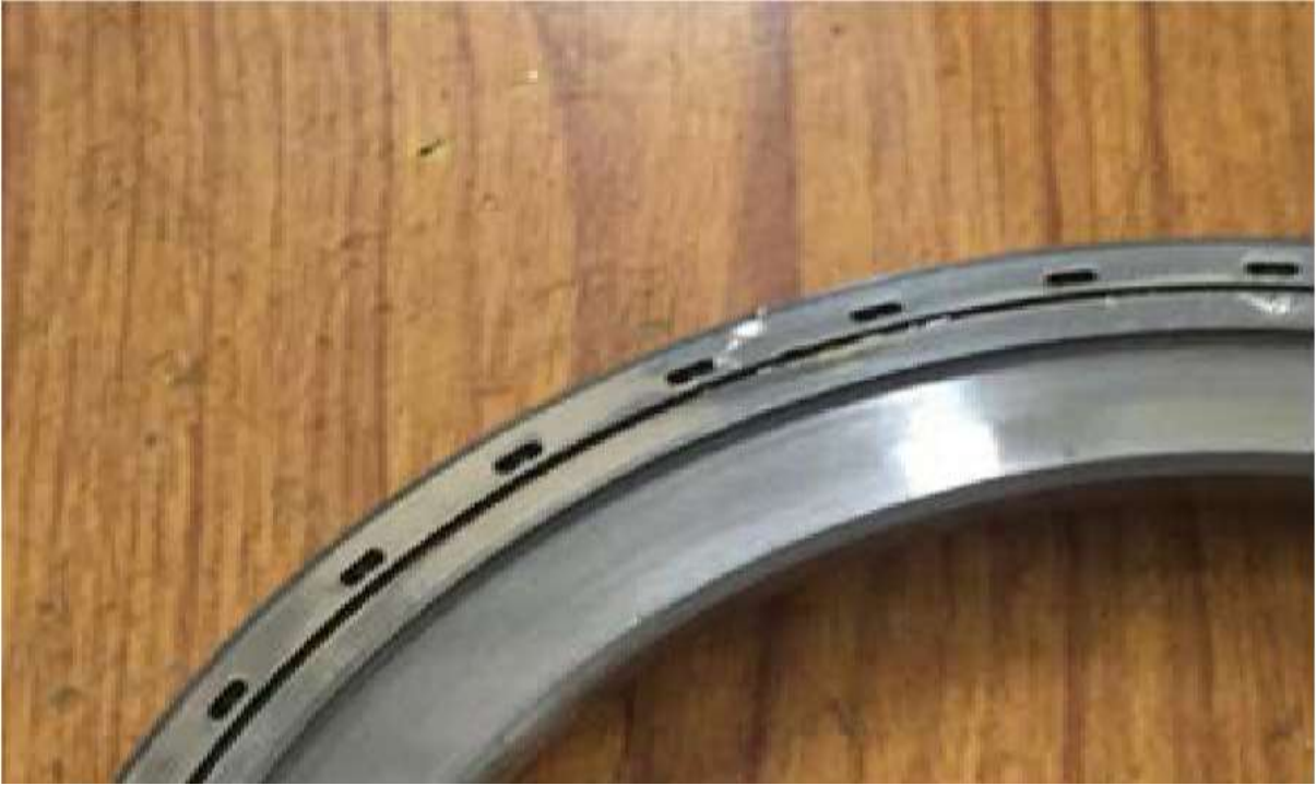
Image #1 – Demonstration seal plate after cleaning and before lapping.
