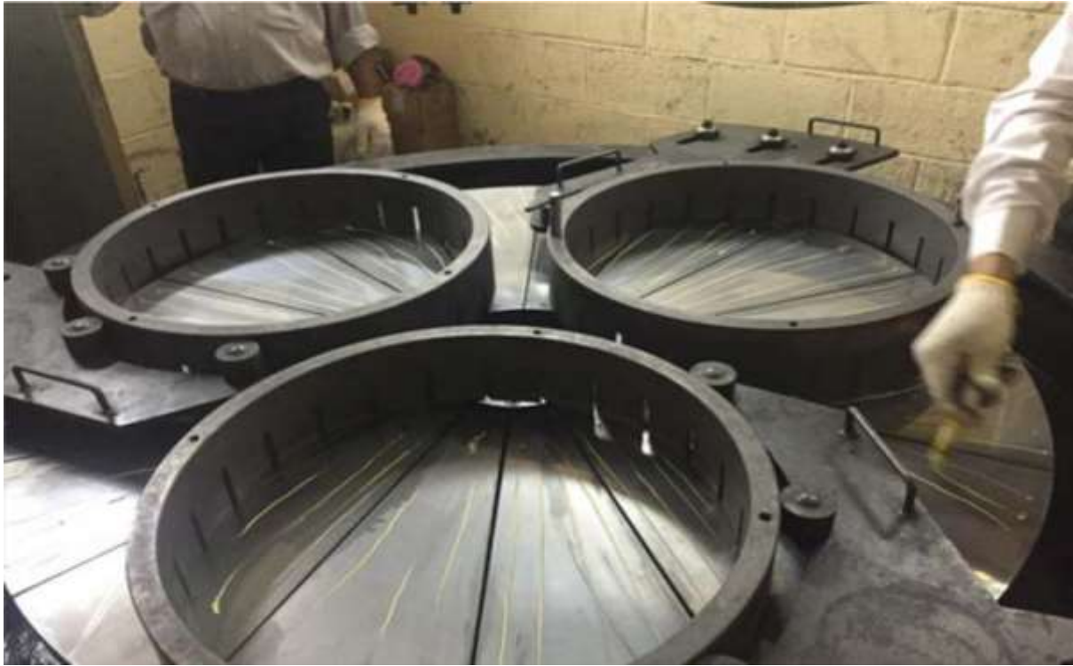
Image #3 - Tooling Installed and Diamond Lapping Paste Applied (yellow streaks).
