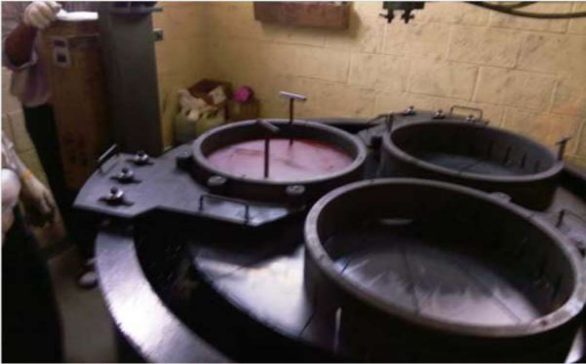
Image #5 – Seal plate installed in lapping machine with 28kg weight installed.
