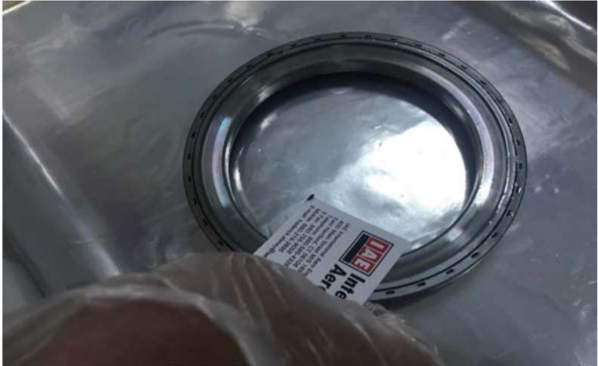
Image #10 – Debris removed from demonstration seal plate after second cleaning cycle.
