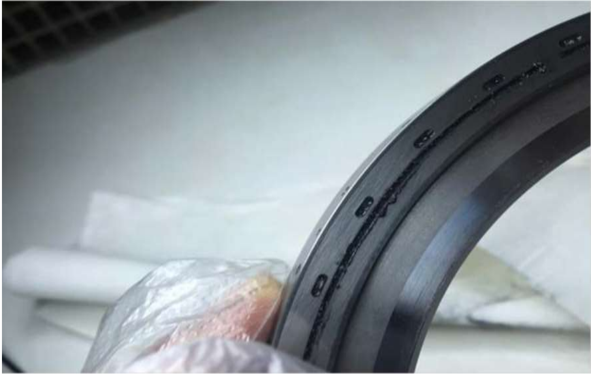
Image #9 – Debris removed from demonstration seal plate groove after process complete.
