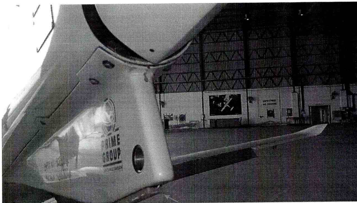
VT-FGA: Rubbing marks on the tail metal skid.
