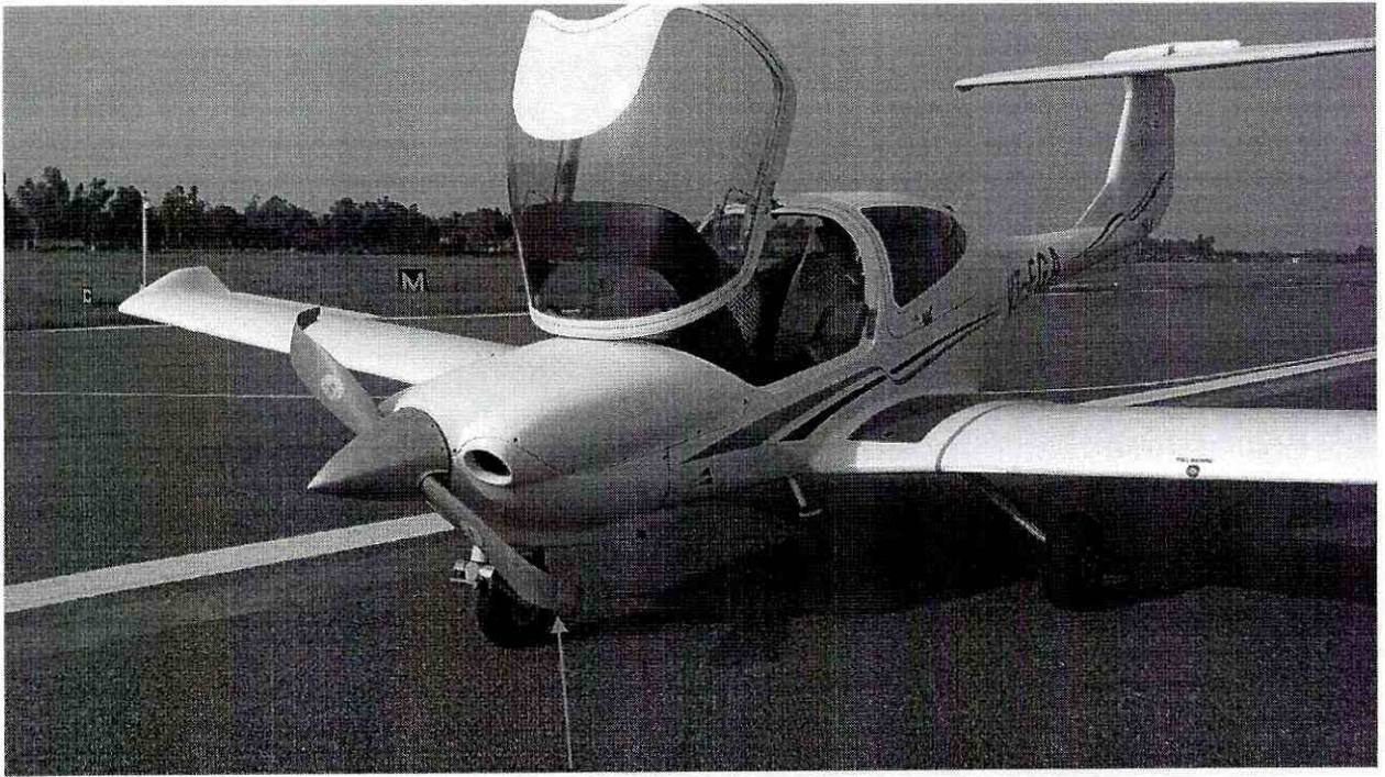
VT-FGA: Both propeller blades bent in propeller strike.
