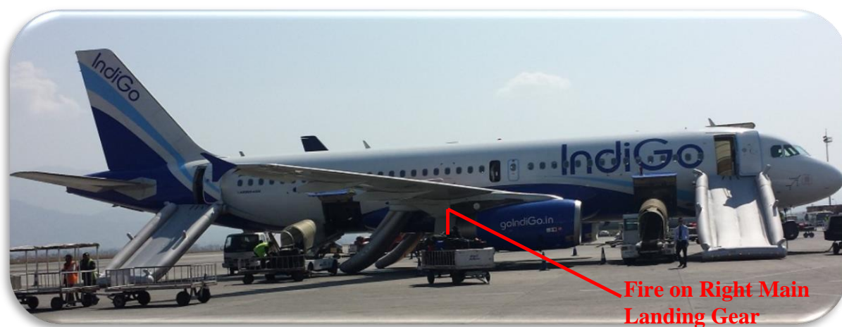
Slides deployed for evacuation
