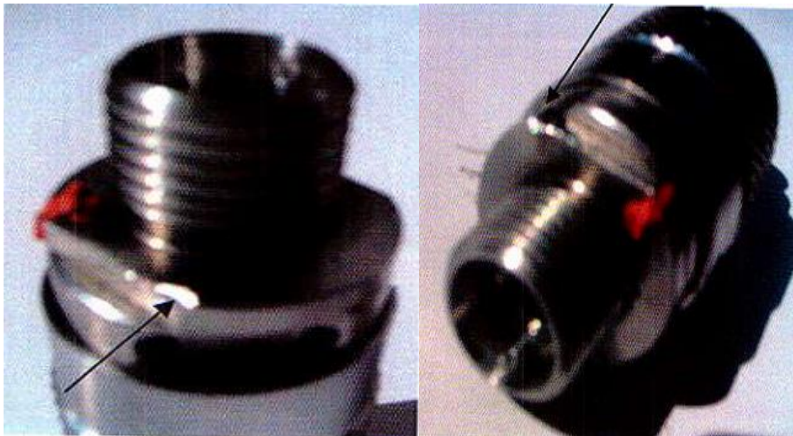
Fig. 5 External Dent marks indicating striking of hard material
