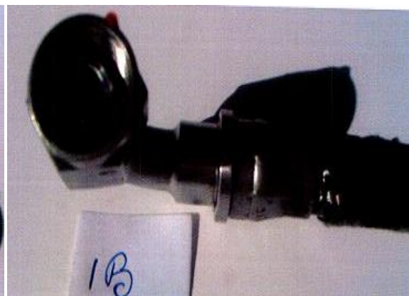
Figure 3b: Shows deep marking on the face of ferrule in the hose pipe
