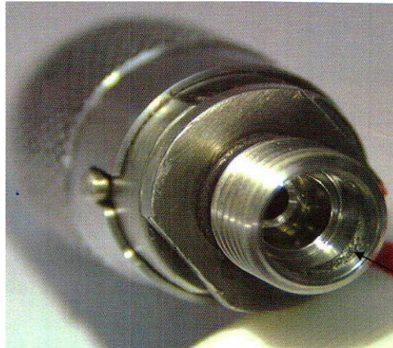
Fig. 4 shows quick release coupling with internal scratches/ metal gauging
