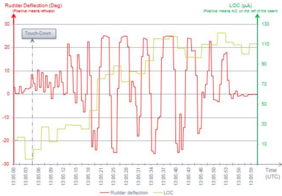
Rudder deflection versus LOC deviation (A/C on the left of the LOC beam)
