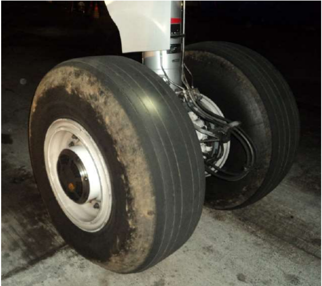
Deflated and damaged tyre (aircraft at parking bay)
