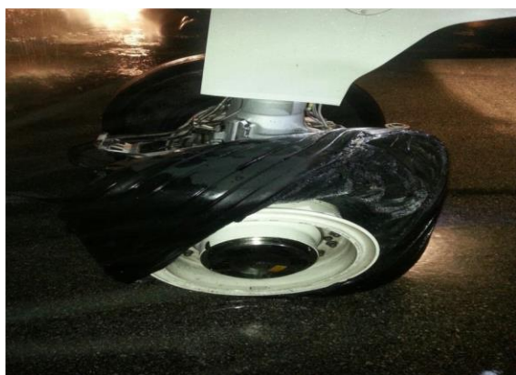
Damaged Right main landing gear wheels
