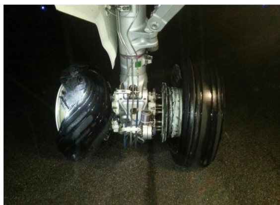
Damaged Right main landing gear wheels
