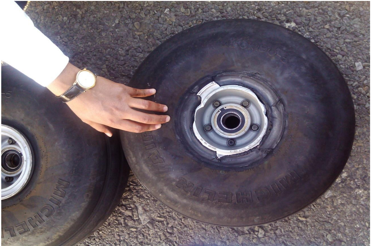
Inner Metal Hub of the Nose Wheel Disintegrated during impact
