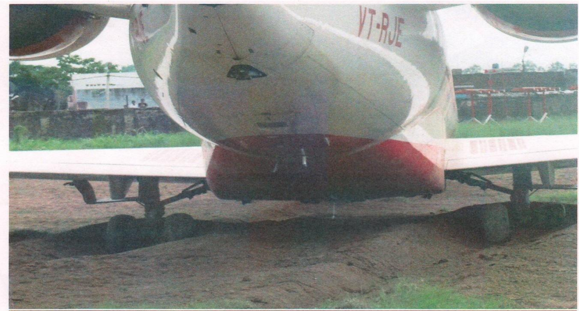
Figure: Both Main Landing Gears Bogged down in soft ground area
