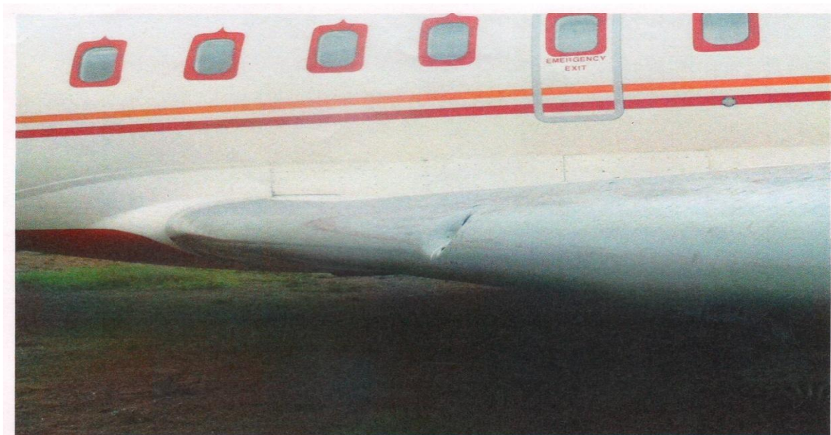
Figure: Damage on the leading edge of the port wing
