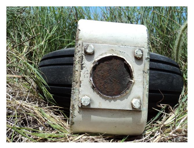
Nose wheel shock strut damaged due to continuous dragging on the runway. No other damage to the aircraft structure was observed. Both the instructor pilot and trainee pilot were safe. No sign of fuel or oil leakage/seepage was observed at the site.
