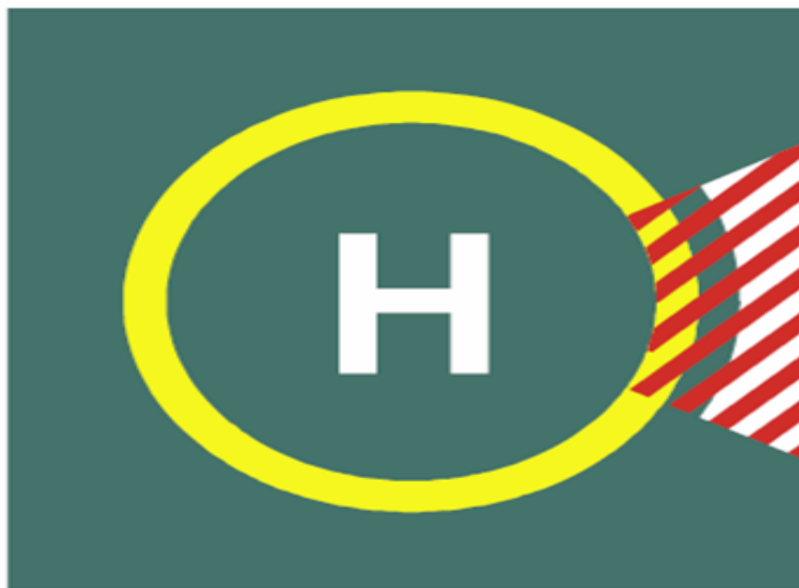
Figure 5-7. Helideck prohibited landing sector marking
